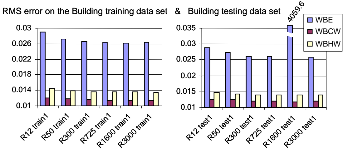
Fig. 6. The error of the GAME ensemble on Building training data decreases with the declining penalization. The results on the testing data set show that no regularization is needed for the WBHW and WBCW variables. For the WBE variable that is much noisier than the other two and for low penalization levels models are overfitted.
